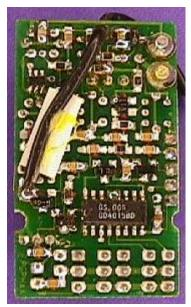
Rear view of 535 circuit board. 16 pin chip between the two notches in the board is the one you want to find.
